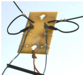
Figure 7 – Antenna end. The thing hanging from the bottom hole is a length of twine used to pull the antenna down to working level.
