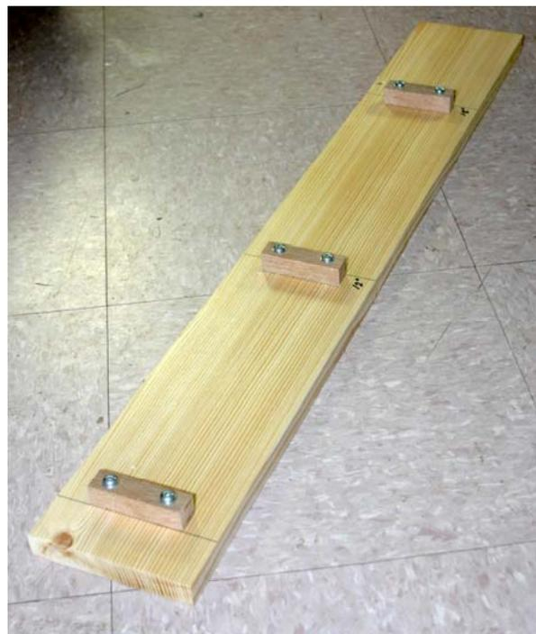
Figure 4 – The spacing jig
