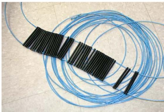
Figure 5 – Plastic spacers on the wire pair
