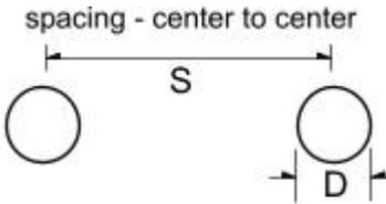
The diagram shows two circles representing wires. A horizontal double-headed arrow above them is labeled "spacing - center to center" and "S". A vertical double-headed arrow below the right circle is labeled "D".
